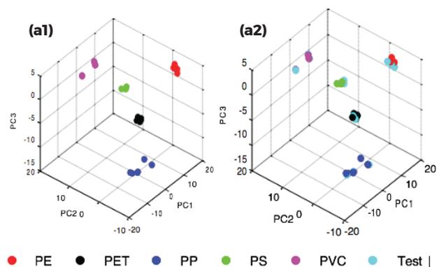
**Figure 2:** The PCA score plots of the first three PCs based on the calibration spectra of the five polymers (a) and the corresponding score plots with the inclusion of the test samples (cyan symbols) (b).
